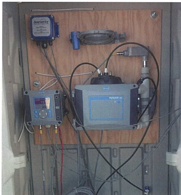
Figure 4-1. Example of EC and Turbidity Instruments used in Pilot Study
